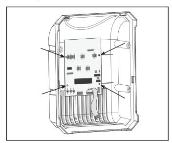
Figure 4. Control PCB Installed
