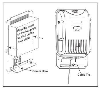
Figure 9. Accessing and Wiring to the Power PCB
