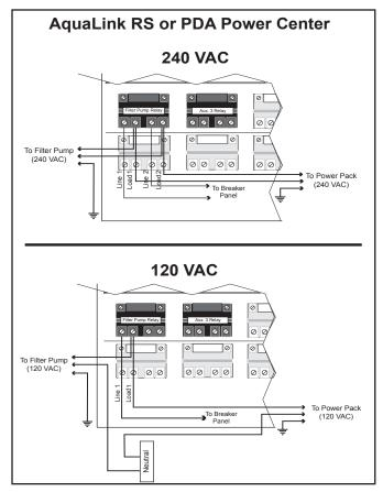
Figure 10. Wiring Power Pack to an AquaLink RS or PDA Power Center (240 VAC and 120 VAC)
