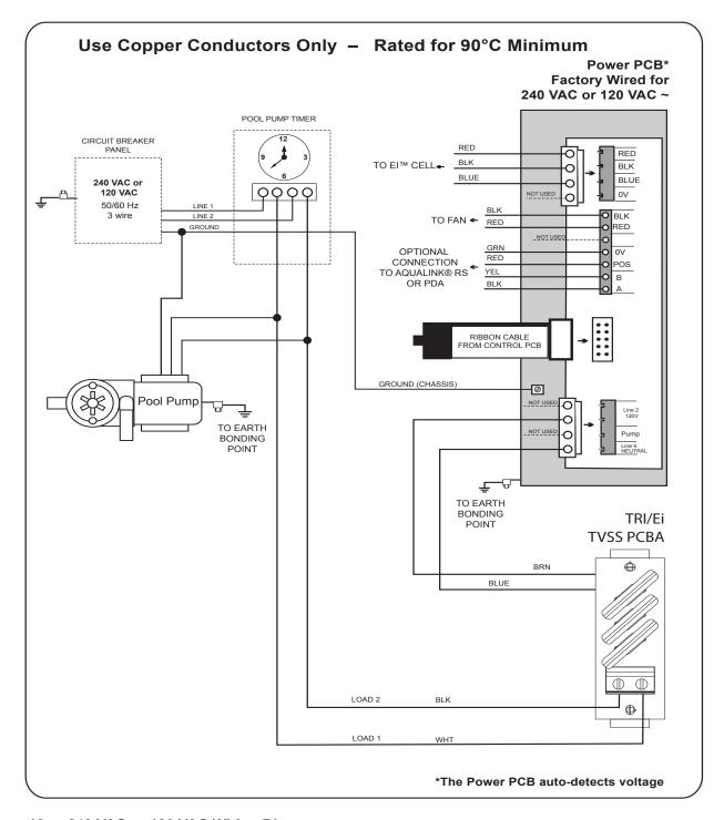
Figure 12. 240 VAC or 120 VAC Wiring Diagram
