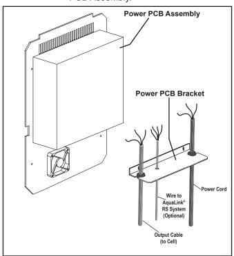
Figure 5. Removing the Power PCB Bracket
