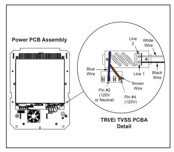
Figure 8. Power PCB with TRI/Ei TVSS PCBA
