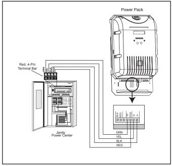
Figure 11. **Communication Wiring between Power** Pack and AquaLink® RS Control System or PDA Network
