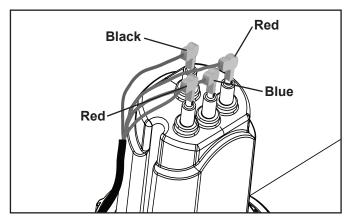
Figure 7. **Connecting Cell Leads**
