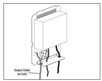
Figure 6. Output Cable Assembly Detached
