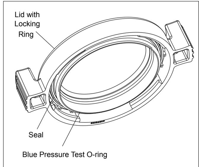
Figure 6: Blue Pressure Test O-ring in Lid Assembly
