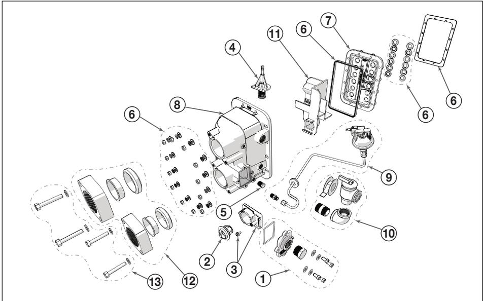
Figure 45. ASME Water System Components
