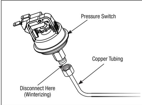
**Figure 25. Water Pressure Switch Copper Tubing (Siphon Tube)**
