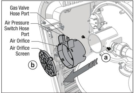
**TIP:** When removing the air hoses from the air orifice, mark the hoses with tape or a marker to help with reassembly.
