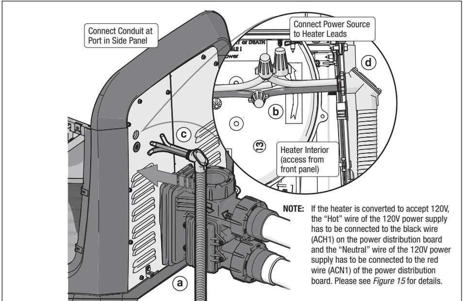
**NOTE:** If the heater is converted to accept 120V, the “Hot” wire of the 120V power supply has to be connected to the black wire (ACH1) on the power distribution board and the “Neutral” wire of the 120V power supply has to be connected to the red wire (ACN1) of the power distribution board. Please see *Figure 15* for details.
