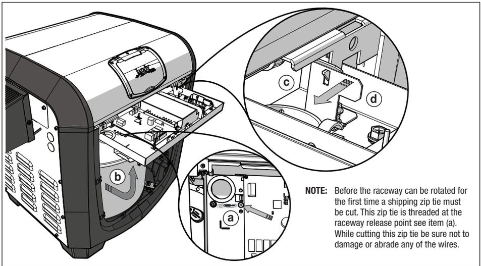
**NOTE:** Before the raceway can be rotated for the first time a shipping zip tie must be cut. This zip tie is threaded at the raceway release point see item (a). While cutting this zip tie be sure not to damage or abrade any of the wires.
