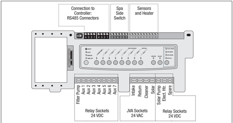
**Figure 21. AquaLink RS PCB with Firmware Rev N or Higher**
