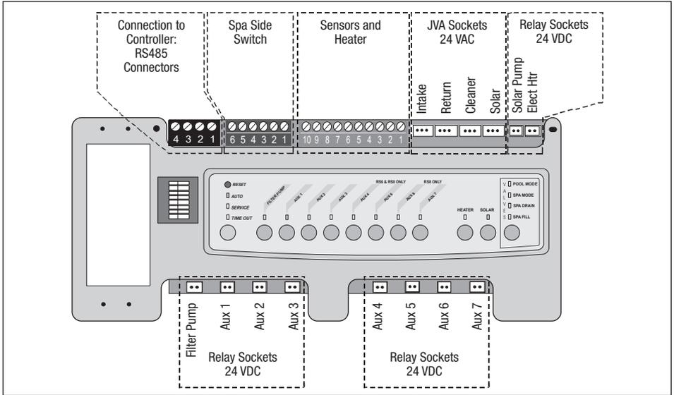
**Figure 20. AquaLink RS PCB with Firmware Rev MMM or Lower**
