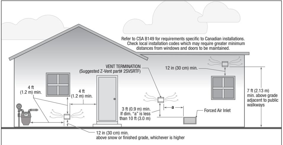
Figure 7. Side Wall Vent Termination
