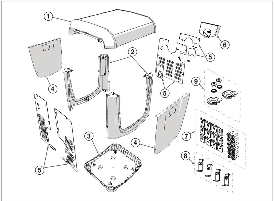
Figure 43. ASME Cabinet Assembly Components
