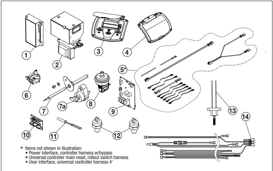
Figure 33. Electrical System Components
