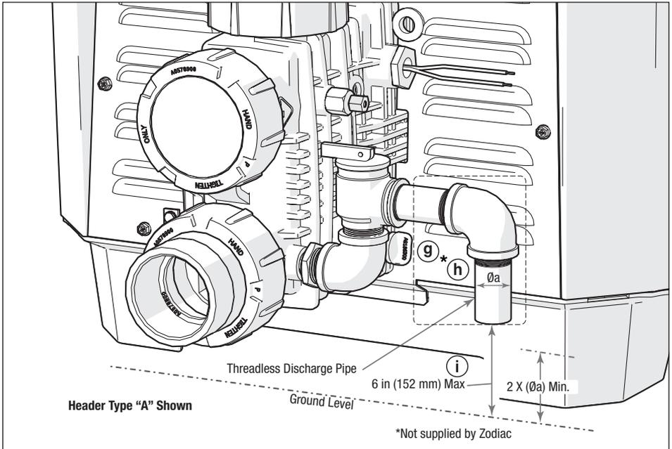
**NOTE:** Hardware showing in dotted line is not provided by Zodiac. Pressure Relief Valve hardware is provided on ASME heater models only.
