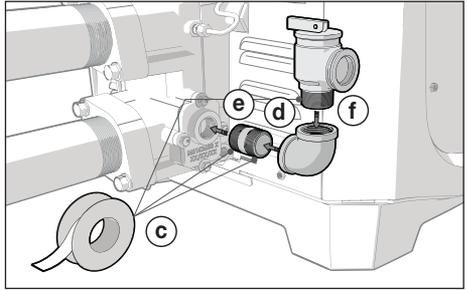
**Figure 41. Install the Elbow**
