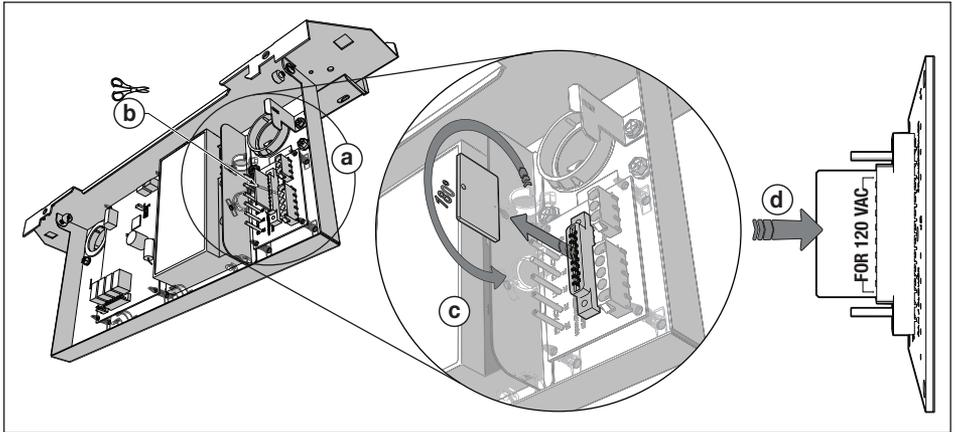
Figure 18. Input Conversion Process
